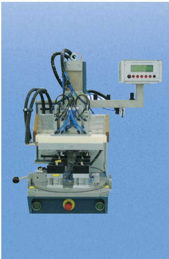
ERW thermal installation machine to embed eight inserts M 1.6 into two mobile phone half shells
